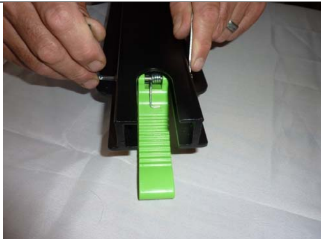
Step 1 – Use the 4mm hex key and the 8mm wrench provided to remove the wheel brake from the scooter.
