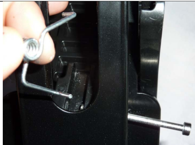
Step 4 – Install the torsion spring into the scooter base and push the spring coil in to line up with the axle bolt..
