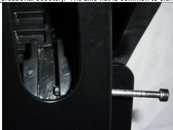
Step 2 – Locate the torsion springs and axle bolts from the kit. Identify the spring and axle bolt for your application (pro or recreational scooter). The axle nut is common to either.
