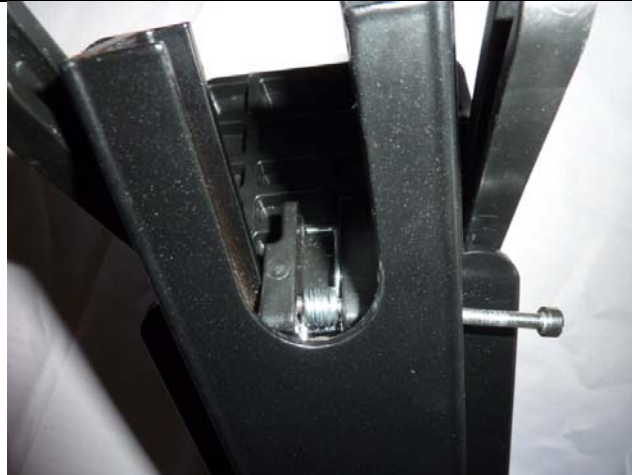
Step 4 – Install the torsion spring into the scooter base and push the spring coil in to line up with the axle bolt..
