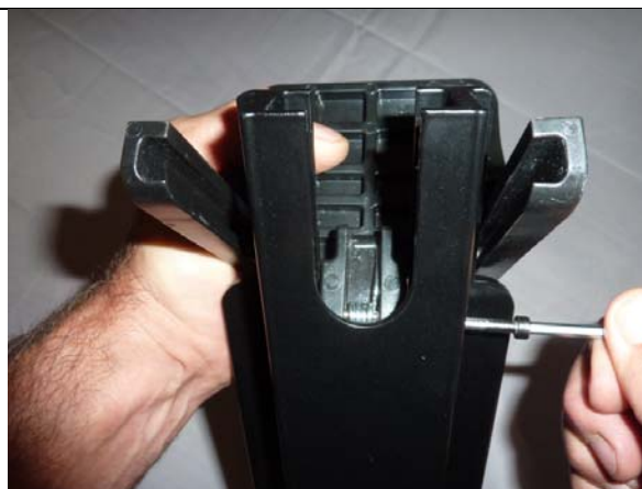
Step 6 – While pulling the brake into proper alignment, push the axle bolt through the axle hole on the far side of scooter base. Install 4mm nut and use the 4mm hex key and the 8mm wrench to tighten the axle snug.
